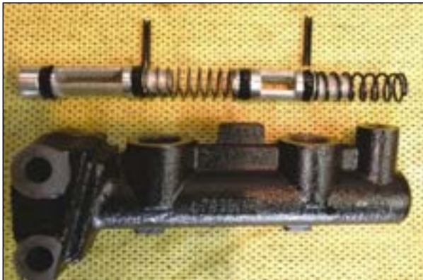
Fig. 2-13 Master cylinder internal components (Courtesy of John Wyers)
